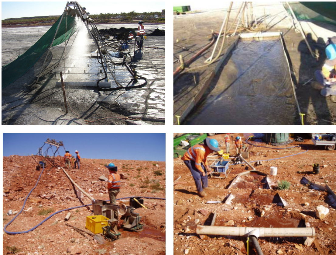
Figure 1.9-1: Rainfall and gully erosion simulations (top is tailings and bottom is growth medium)
