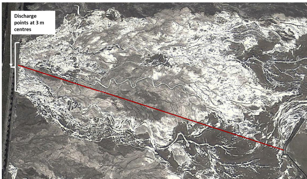
Figure 2 Meandering flow from 30 simultaneously operated discharges at 3 m centres and a beach length of 740 m
